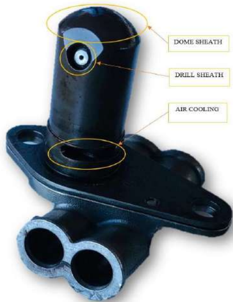
Fig. 5: Fuel injector with head sheath.
