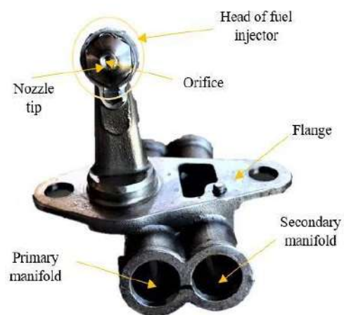
Fig 4: Fuel injector without head sheath.
