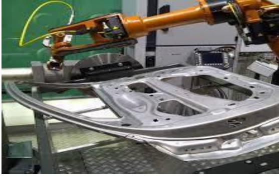
Fig 8. Remote Welding in Automotive Industry. [7]
