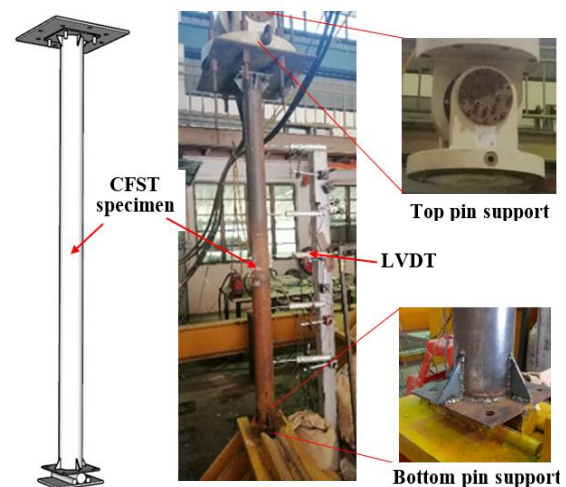
Fig 6. Test setup of the CFST Long columns.
