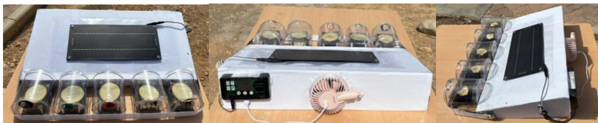
Fig 5. The hybrid solar dryers design for improved heat and mass transfer.
