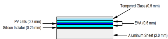
Fig 3. Schematic diagram for silicon isolator PV panel.
