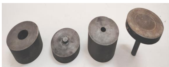
Fig 3. Photograph of the machined compaction die with the ejector piece (left) used to remove the compacted specimens.
